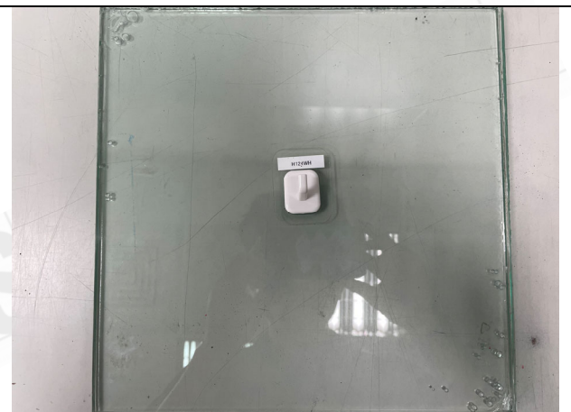
Photo D: After Oven Test- Self Adhesive Hooks-front
